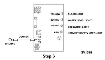
Jumper wire connected from control board terminal 1F to ground Is water flowing **The Water Inlet** The Water Level into the water Valve Solenoid Cause Light is: trough? Coil is: The water level probe is causing the problem. De-Energized no on Clean or replace the water level probe. off Energized The control board is causing the problem. yes De-Energized The water fill valve is causing the problem. yes on
